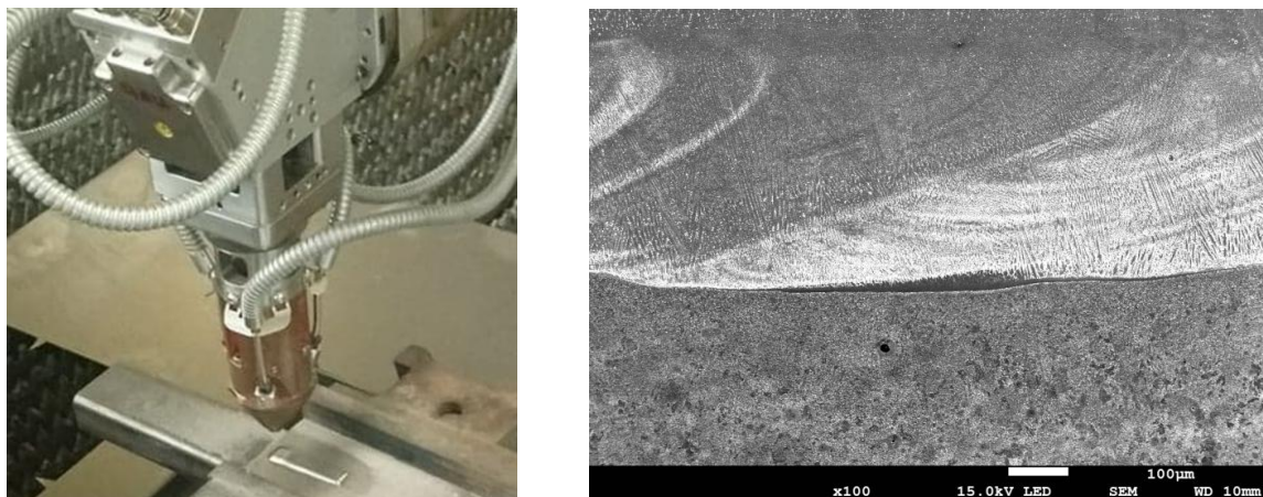
Fig. 6. Laser cladding process using powder (left) and SEM image of clad layers on a cross-section (right)
