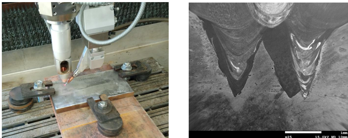
Fig. 5. Laser cladding process using wire (left) and SEM image of clad layers on a cross-section (right)
