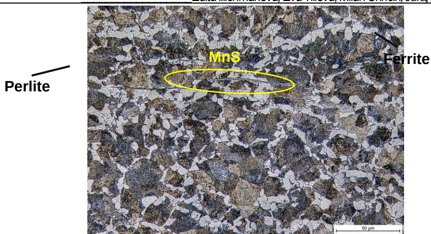
Fig. 1. Detail of the microstructure of the sample in its initial state, etched with 3% Nital
