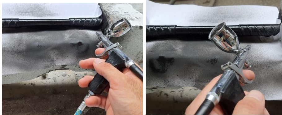
Fig. 6. Application of speckles on the working reinforcement using an airbrush
