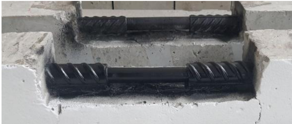
Fig. 3. View of the opening in the tested beams for access to the tensile reinforcement when using the DIC method
