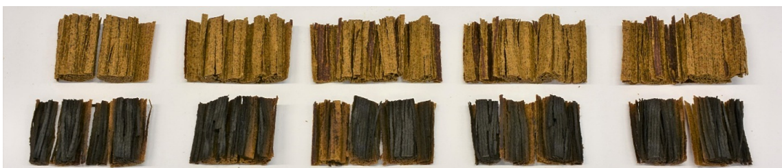
Figure 7. Optical photographs of tobacco portions extracted from unused EHTPs (top row) and used EHTPs (bottom row) for five replicates.
