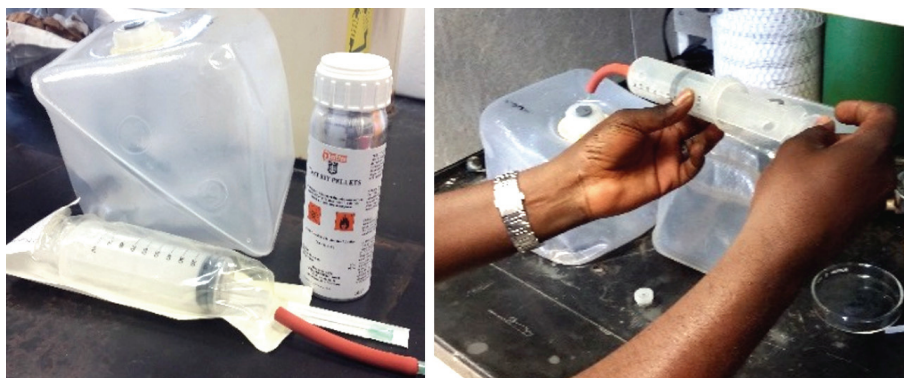
Figure 5. The Degesch™ phosphine tolerance test kit (left) ( https://detia-garda.de/wp-content/uploads/2019/05/Phosphine-Tolerance-Test-Manual.pdf ). The kit includes two small pellets of magnesium phosphide, a 3.7-L plastic water jug in which the pellets are reacted with a small amount of water to generate an atmosphere of 6,000 ppm phosphine (left image). A small group of beetles are placed in a large see-through plastic syringe before a blend of gas and air is added to the barrel to result in a concentration of 3000 ppm phosphine. Beetles are observed for 30 min to count the number of susceptible beetles that are knocked-down by the phosphine. Beetles that remain upright and appear normal are scored as resistant.
