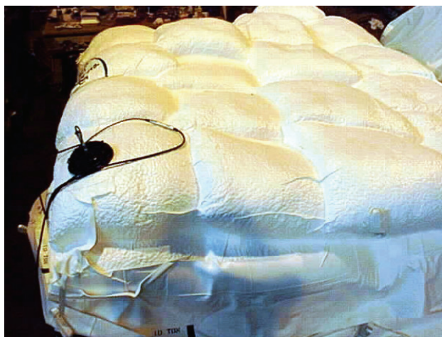
Figure 7. A GrainPro cocoon containing bagged commodity subjected to a low oxygen atmosphere using a vacuum pump to achieve approximately 1% oxygen. The same gas-tight covering could be used for tobacco under low O 2 (via vacuum or high N 2 ), high CO 2 , or a small application of a fumigant.
