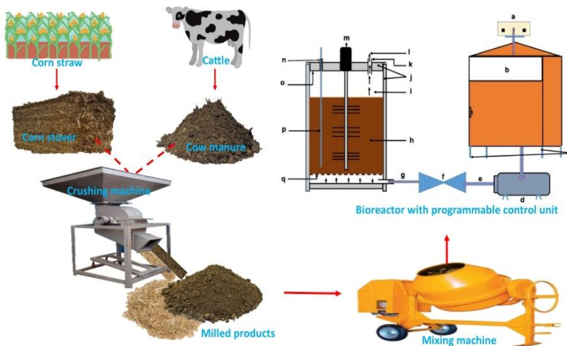
Figure 2. Graphical representation of the bioreactor components and the composting process: (a) switch; (b) programmable control unit (PCU); (c) stand, (d) gas cylinder; (e) gas supply line; (f) automatic point of oxygen regulation, (g) inlet valve; (h) feedstock; (i) reactor headspace; (j) insulator; (k) outlet valve; (l) point of gas collection; (m) rotator; (n) point of thermometer fixation; (o) reactor lid; (p) thermometer; and (q) seal liner
