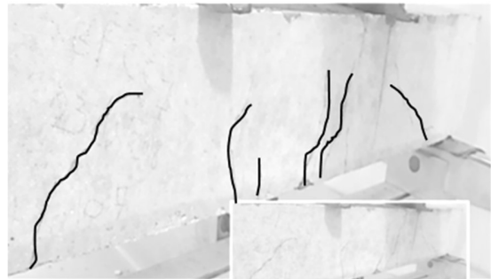
(d) Beam with crimped steel fibers (BC-1.05): Flexural-Shear Failure
