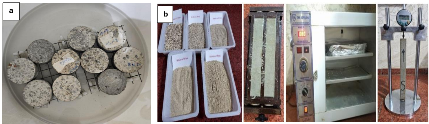
Figure 9: Durability test setup: (a) Sorptivity, and (b) Alkali-silica reaction (ASR) expansion
