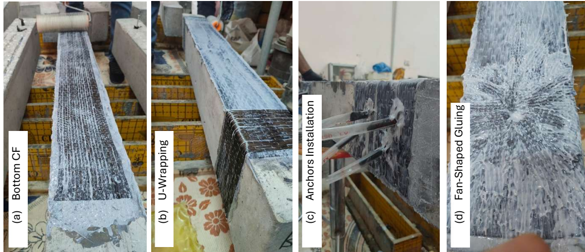
Figure 7: Strengthening and anchoring test specimens using CF sheets, u-wrapping and spike anchors
