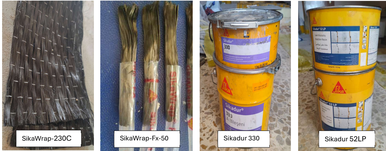
Figure 2: Carbon fibre and epoxy materials used in this research
