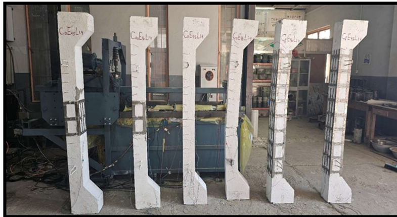
Figure 14: Failure of all columns
