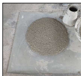
(a) slump flow and T500 test
