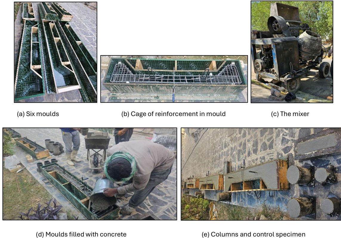
Figure 3: Casting process of concrete
