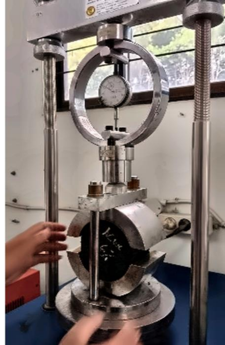
(c) Marshall stability and flow testing
