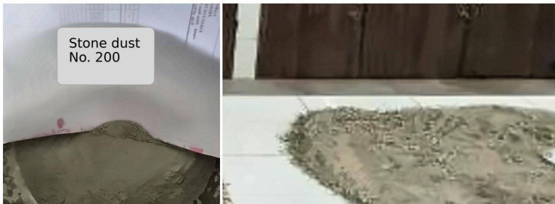
Figure 2: Fine materials used in the study: (a) stone dust and (b) Kampar River sand
