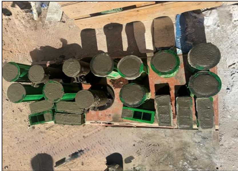
Figure 4: Small foamed concrete specimen cast for laboratory testing
