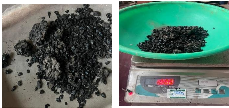
Figure 3: Reclaimed Asphalt Pavement (RAP) particles showing aged asphalt coating and granular morphology used for preparing RAP–soil mixtures.
