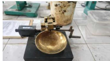
(b) Liquid limit test using Casagrande apparatus
