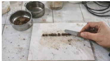
(c) Plastic limit determination by manual rolling method
