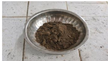
(a) Natural soil sample prepared for Atterberg limits testing
