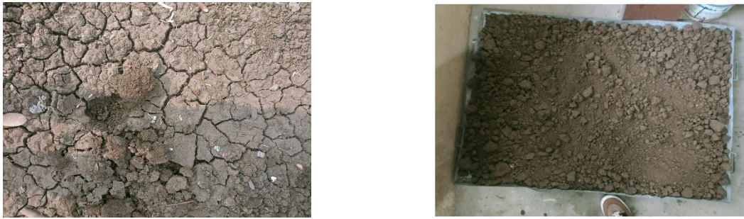
Figure 2: Natural soil sample collected for laboratory characterization prior to index property and compaction testing
