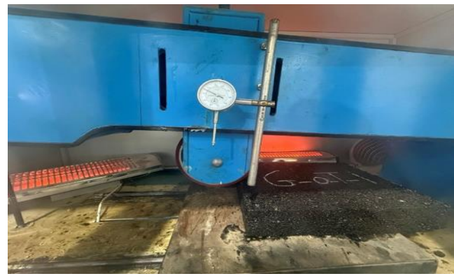
(b) Slab conditioning
