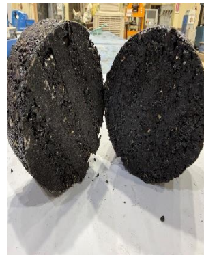
(c) Some of the failed specimens after testing
