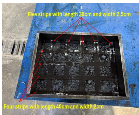
(d) Tack coat and 50% geotextile as interlayer
