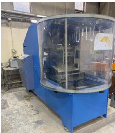
(a) Roller compactor device
