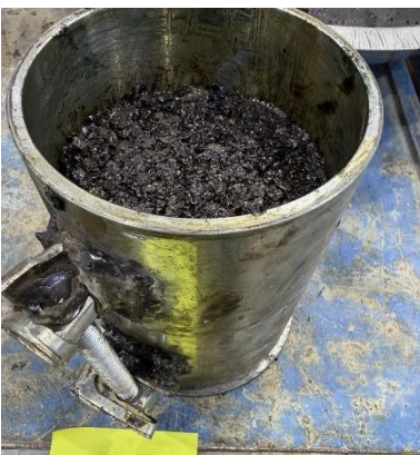
(g) Two-layer sample in the mold
