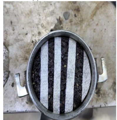
(f) 50% geotextile as interlayer
