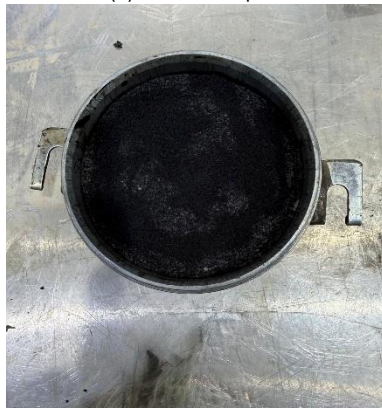
(e) Tack coat and 100% geotextile as interlayer
