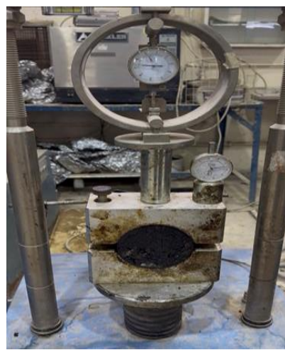
Figure 4: Marshall specimens testing
