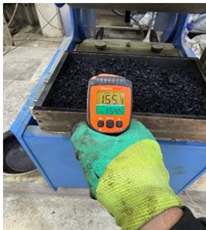
(b) HMA in the mold
