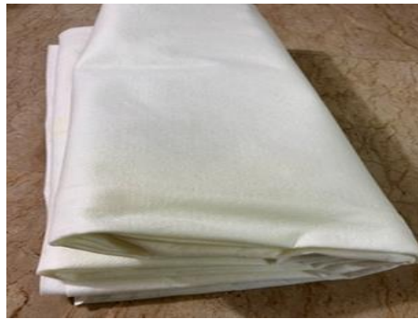
Figure 2: Nonwoven Polypropylene Geotextile paving fabric used in this study
