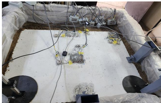
Figure 5: Concrete slab in a laminar box on a shaking table
