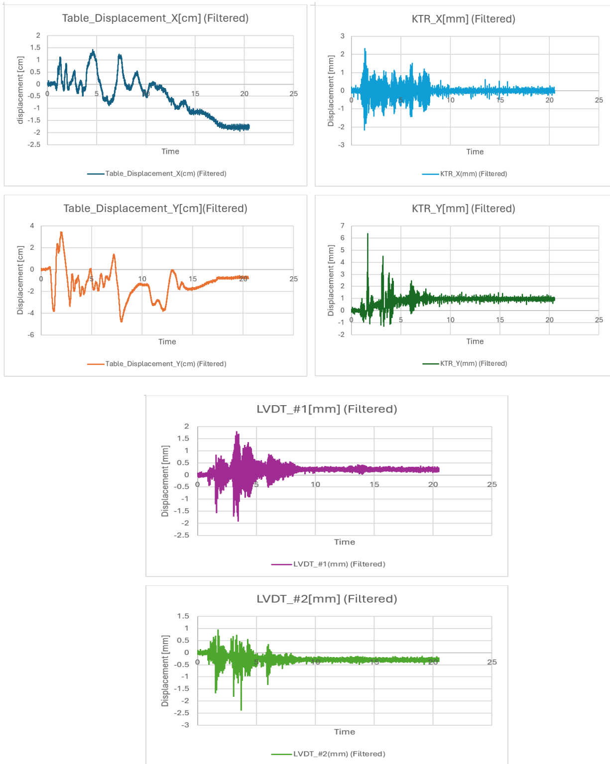
Figure 6: Displacement tests of shaking table: (a) NC samples; (b) PPF sample; (c) SF Sample; (d) HF sample
