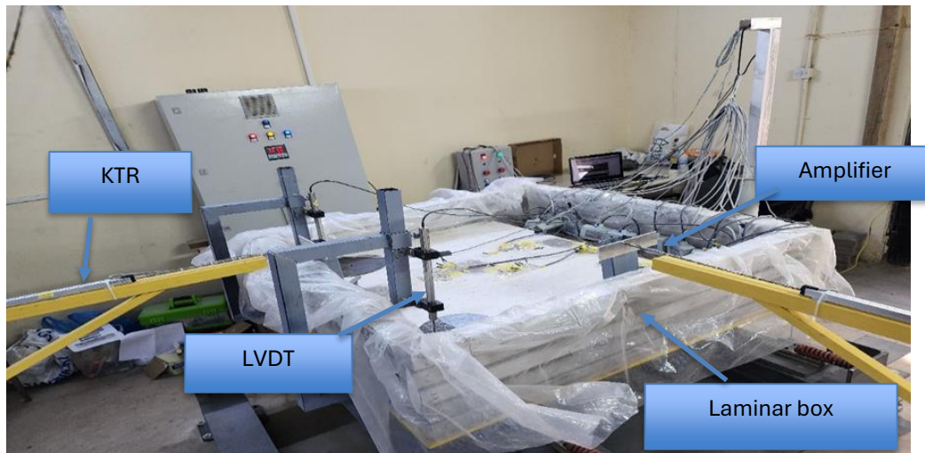
Figure 4: Test set-up and details of the instrumentations
