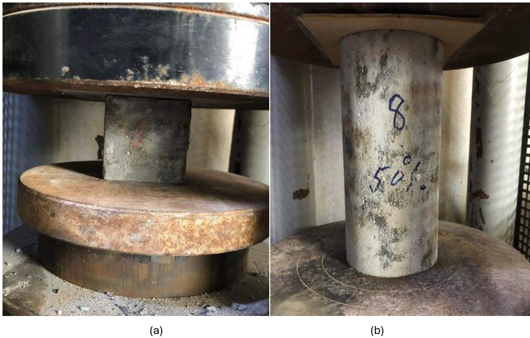
Figure 6: Compressive strength test of (a) cube specimen, (b) cylindrical specimen
