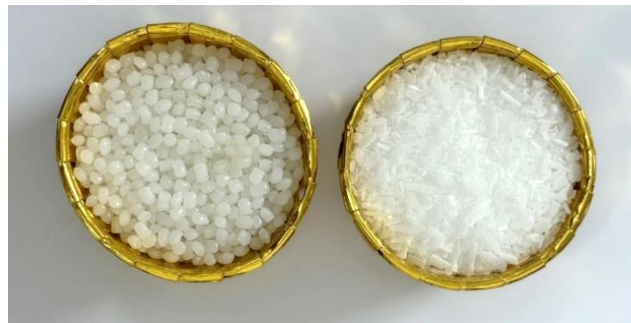
Figure 2: SBS modifier (left) and PEG modifier (right)
