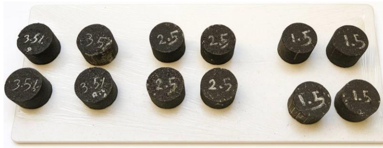
Figure 4: Some of prepared specimens for splitting test
