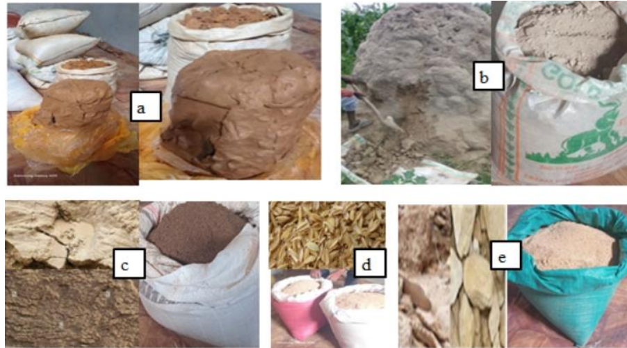
Figure 1: Raw materials; (a) clay, (b) termite mound soil, (c) river sand (d) rice husk, and (e) lime
