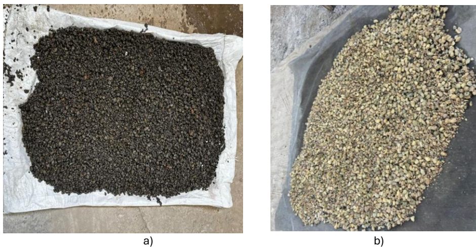
Figure 1: Lightweight Coarse Aggregates: a) LECA; b) ATG
