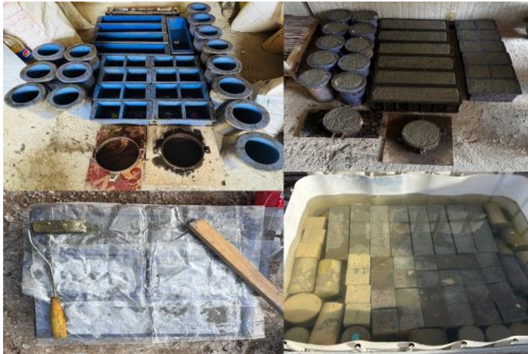
Figure 4: Casting and Curing Of LWSCC Mix
