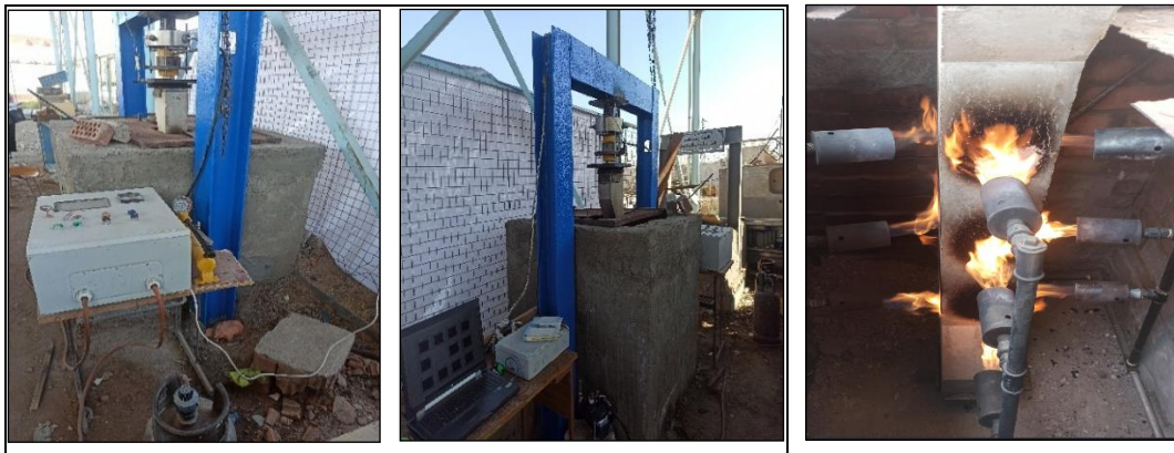
Figure 4: Specimens subjected to fire exposure under pre-loading curve
