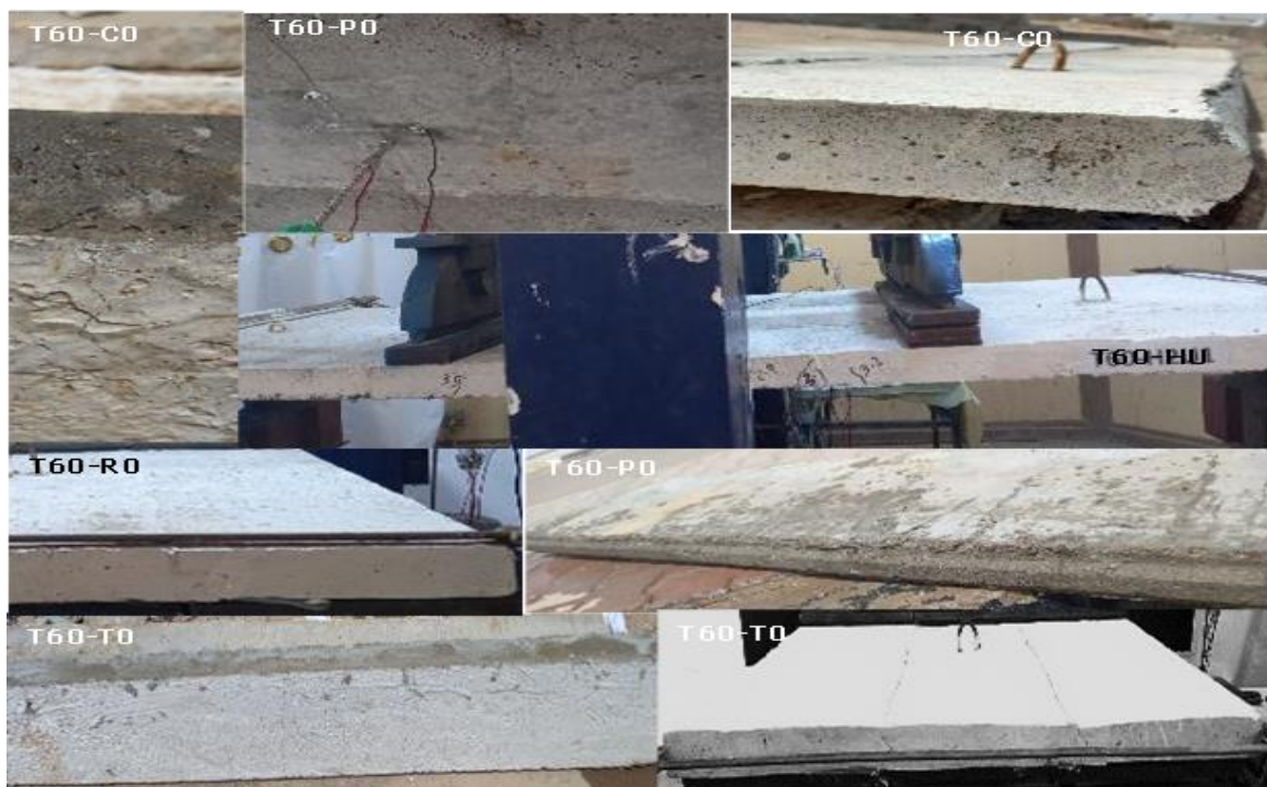
Figure 21: Failure Mode of specimens
