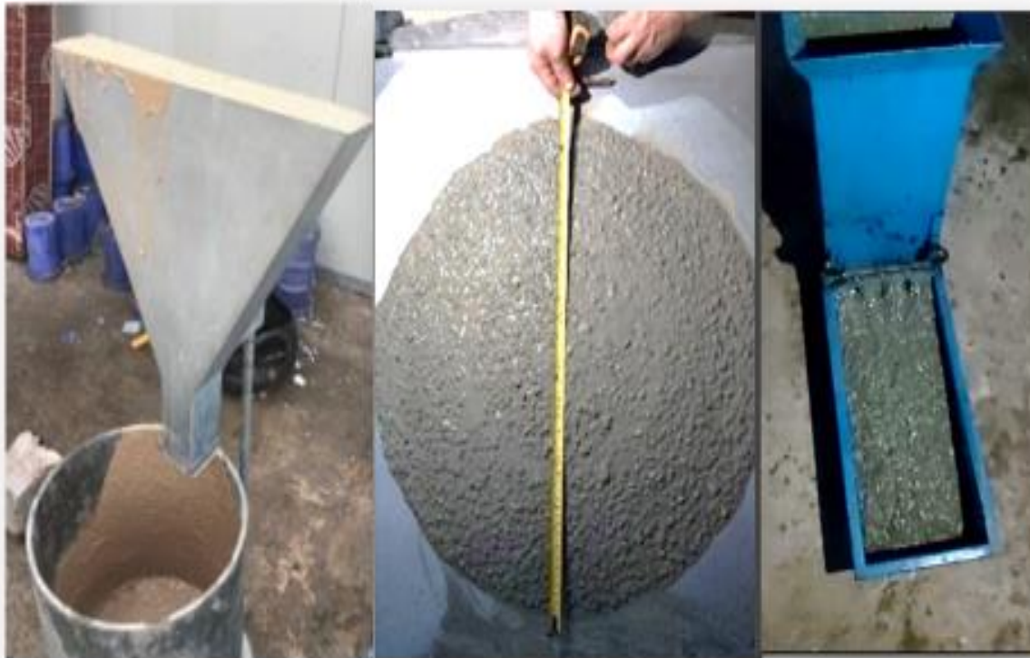
Figure 4: V-funnel, slump flow and L-box tests of fresh concrete
