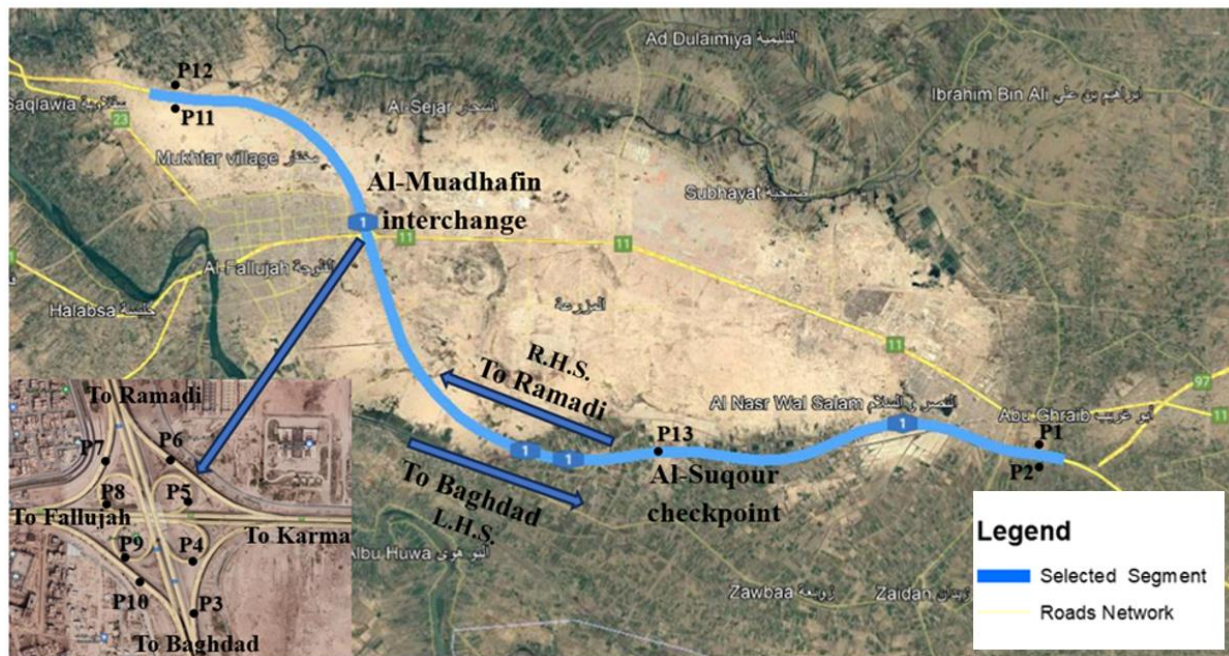
Figure 3: Traffic counting stations
