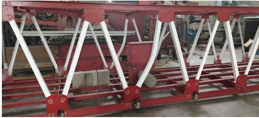
Figure 13: Experimental simulation of mid-span diagonal member damage (Dmg-BC)
