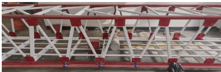
Figure 25: Experimental simulation of diagonal member damage at 1/5 of the span (Dmg-EE)
