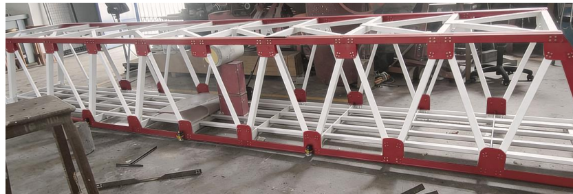
Figure 16: Experimental simulation of mid-span diagonal member damage (Dmg-EC)
