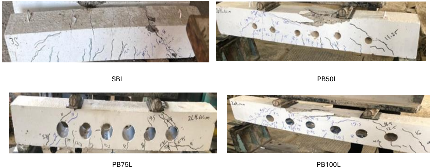
Figure 5: Experimental crack patterns in beams at failure
