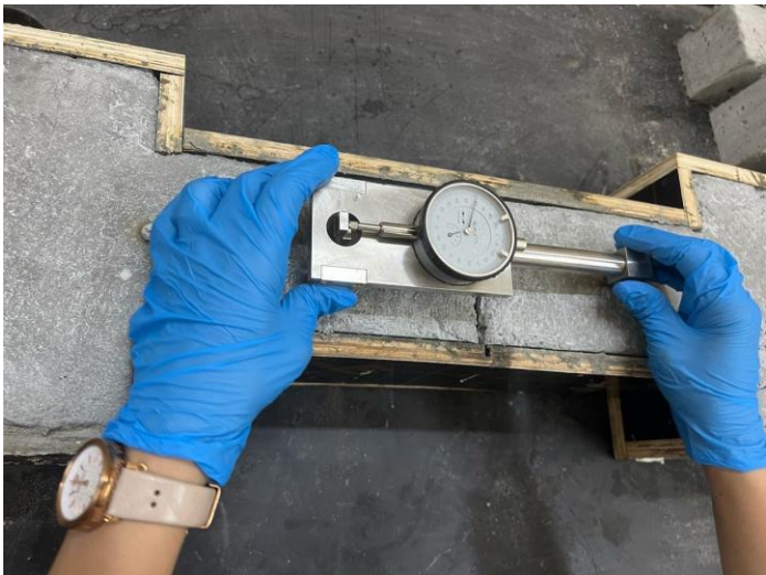
Figure 4: I-shaped specimen with central groove and Demec points, showing the autogenous shrinkage test setup using a mechanical extensometer
