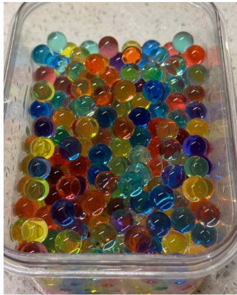
Figure 1: Water absorption polymer balls (WAPB) in concrete mixes
