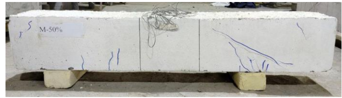
b) Failure mode of a 50% pre-damaged beam (M-50%)
