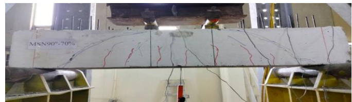
h) Failure mode of a 70% pre-damaged beam strengthened by CFRP bars at 90° near longitudinal reinforcement (MSN90-70%)
