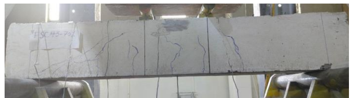
j) Failure mode of a 70% pre-damaged beam strengthened by CFRP bars at 45° in the center (FSC45-70%)
