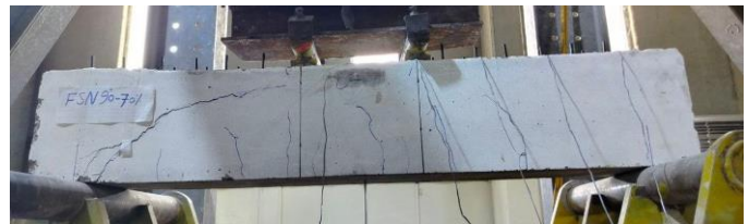
d) Failure mode of a 70% pre-damaged beam strengthened by CFRP bars at 90° near longitudinal reinforcement (FSN90-70%)
