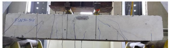
h) Failure mode of a 50% pre-damaged beam strengthened by CFRP bars at 90° near longitudinal reinforcement (FSN90-50%)
