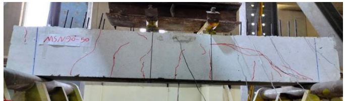
d) Failure mode of a 50% pre-damaged beam strengthened by CFRP bars at 90° near longitudinal reinforcement (MSN90-50%)
