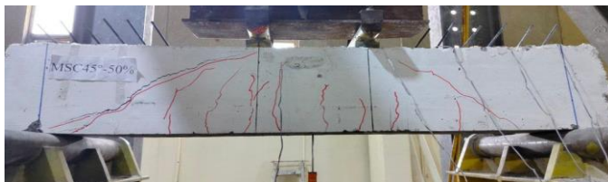
e) Failure mode of a 50% pre-damaged beam strengthened by CFRP bars at 45° in the center (MSC45-50%)
