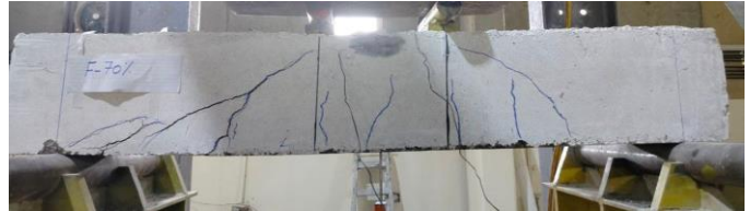
b) Failure mode of a 70% pre-damaged beam (F-70%)
