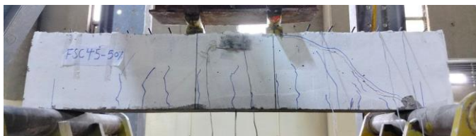
i) Failure mode of a 50% pre-damaged beam strengthened by CFRP bars at 45° in the centre (FSC45-50%)
