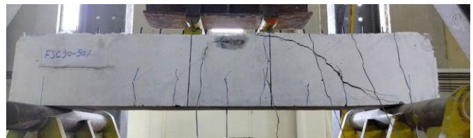
f) Failure mode of a 50% pre-damaged beam strengthened by CFRP bars at 90° in the center (FSC90-50%)
