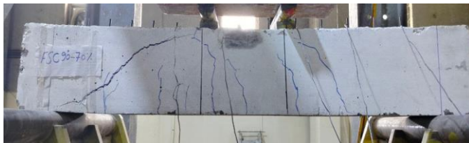
g) Failure mode of a 70% pre-damaged beam strengthened by CFRP bars at 90° in the center (FSC90-70%)
