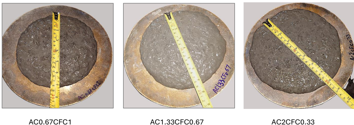
Figure 6: The degrees of distortion in the matrices that were put through the mini-slump flow test
