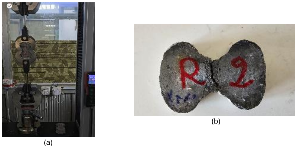
Figure 1: Dog-bone specimens of SC-ECC mixtures under direct tensile test: (a) specimen mounted in the testing machine during loading, and (b) specimen after failure showing the final dominant crack and residual fine cracks within the gauge length
