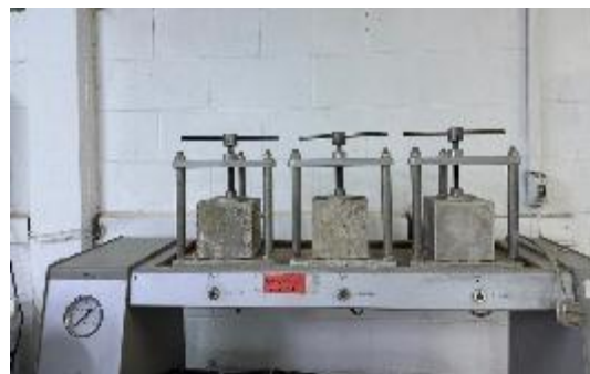
Figure 4: Water permeability test setup for SC-ECC specimens under 0.5 MPa hydrostatic pressure, results evaluated according to DIN 1048-5 (1991)
