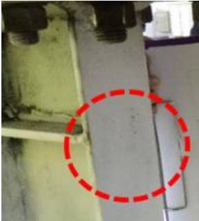
Figure 13(a), Yield initiation: paint flaking observed at the stiffener-proximate flange (specimen LL-0, 5A Cycle).
