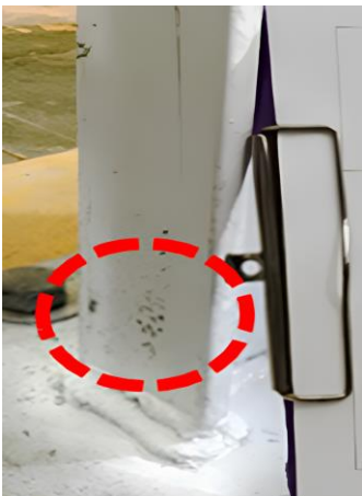
Figure 13(g), Yield condition: paint flaking observed at stiffener-proximate flange (specimen LL-2, 6B Cycle).
