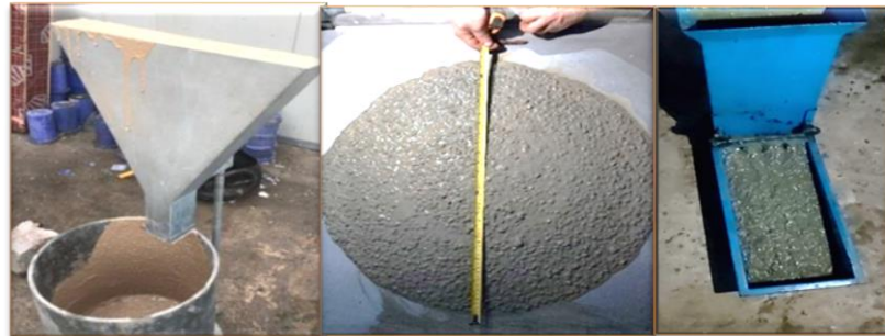
Figure 4: V-funnel, slump flow and L-box tests of fresh concrete
