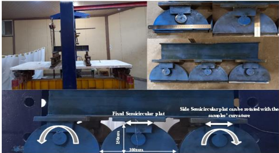
Figure 7: Experimental Loading Setup System
