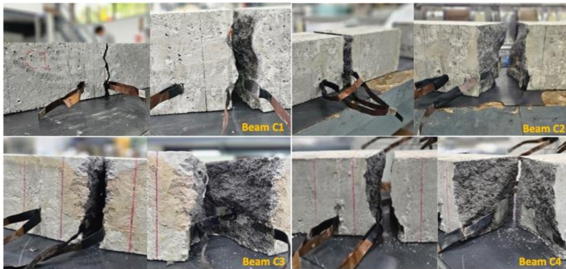
Figure 7: Final damage condition of the tested beam after four-point bending failure
