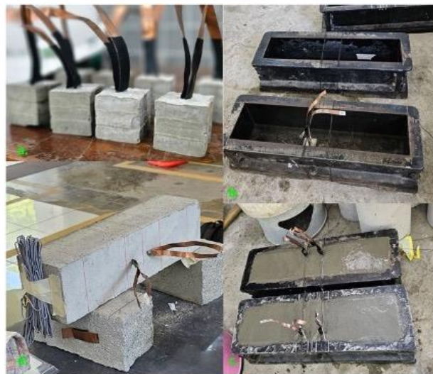
Figure 3: Sensor and beam preparation
