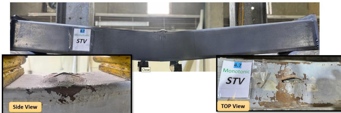
Fig. 15b: Failure behaviour of STV beams with vertical notches in the compression zone with thickness 4.7.
