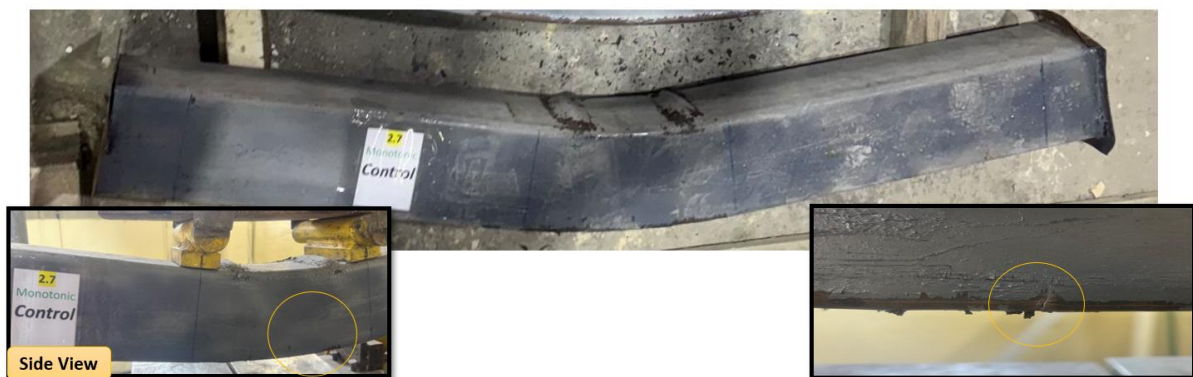
Fig. 14a: Failure Behaviour of Control Steel Tube Beams with thickness 2.7.
