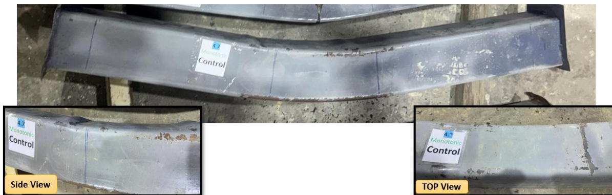
Fig. 14b: Failure Behaviour of Control Steel Tube Beams with thickness 4.7.
