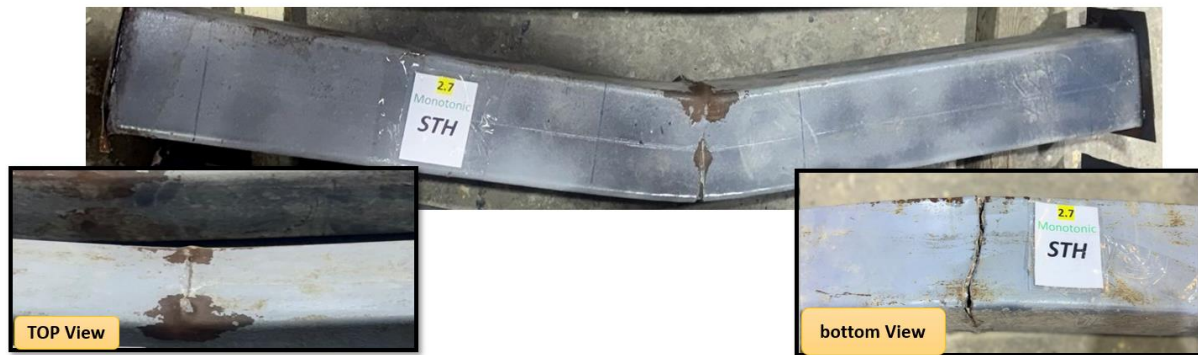
Fig. 16a: Failure behaviour of STH beams with horizontal notches in the compression zone with thickness 2.7.
