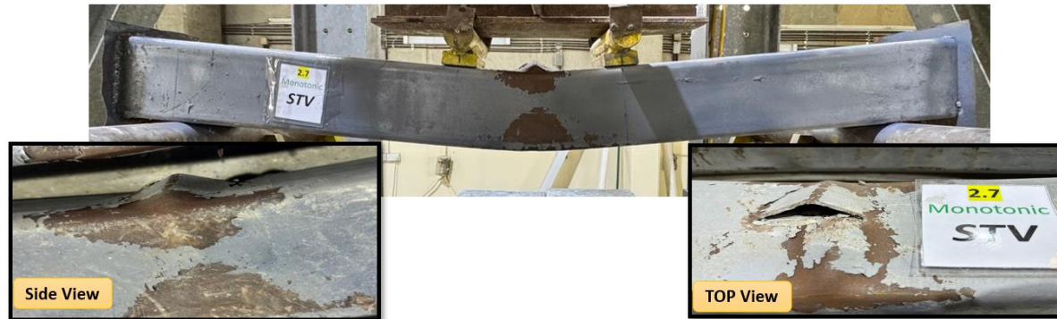
Fig. 15a: Failure behaviour of STV beams with vertical notches in the compression zone with thickness 2.7.
