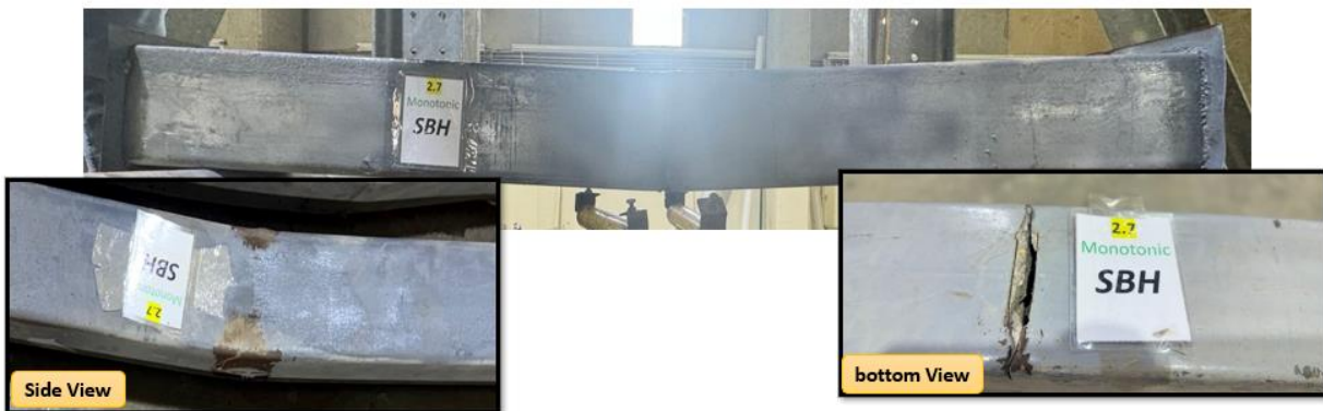
Fig. 18a: Failure behaviour of SBH beams with horizontal notches in the tension zone with thickness 2.7.
