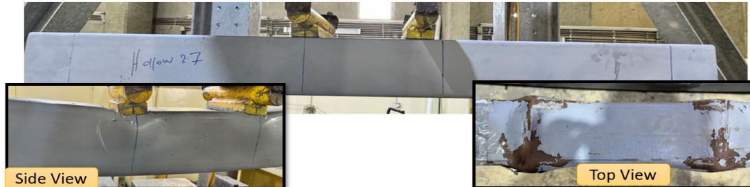
Fig. 13a: Failure Behaviour of Hollow Steel Tube Beams with thickness 2.7.
