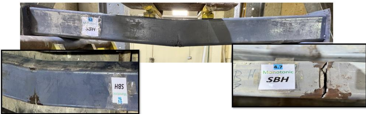
Fig. 18b: Failure behaviour of SBH beams with horizontal notches in the tension zone with thickness 4.7.
