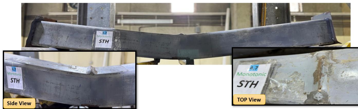
Fig. 16b: Failure behaviour of STH beams with horizontal notches in the compression zone with thickness 4.7.
