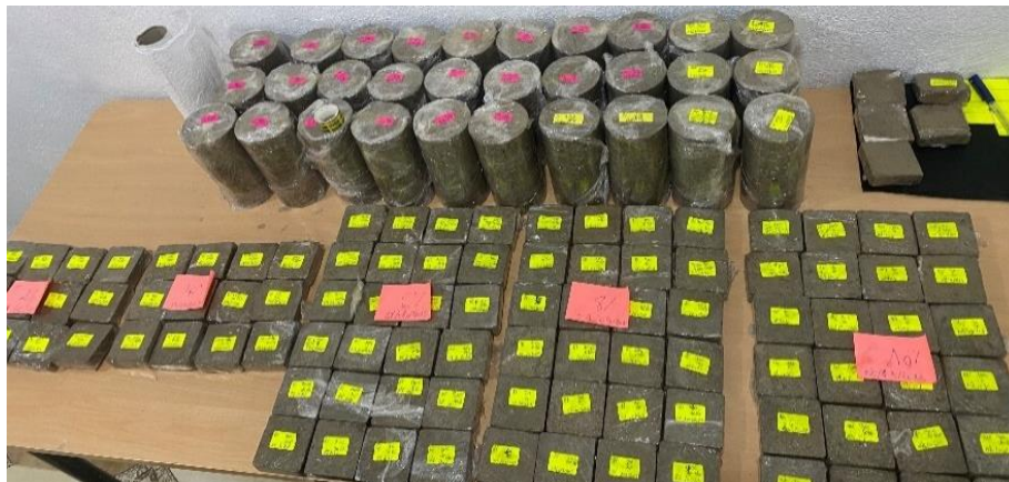
Fig. 3: Photo of specimens prepared for UCS and shear tests.
