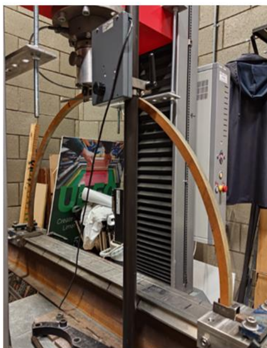
Fig. 4: Experimental measurement of the arch with a radius of 500 mm, component details.
