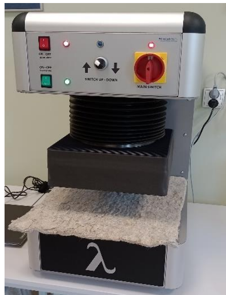
Fig. 3: Heat Flow Meter LM.PLUS 305.
