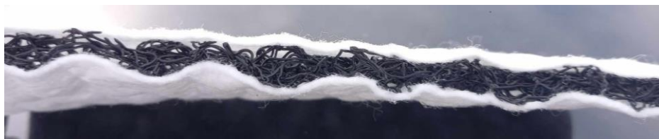
Fig. 2: Test sample (drainage geocomposite MacDrain® W 1071 I).
