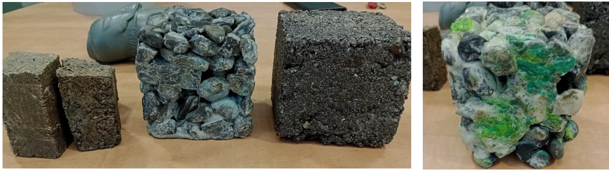
Fig. 1: Samples produced at the University of Bielsko-Biala from a mixture of melted plastic and gravel.
