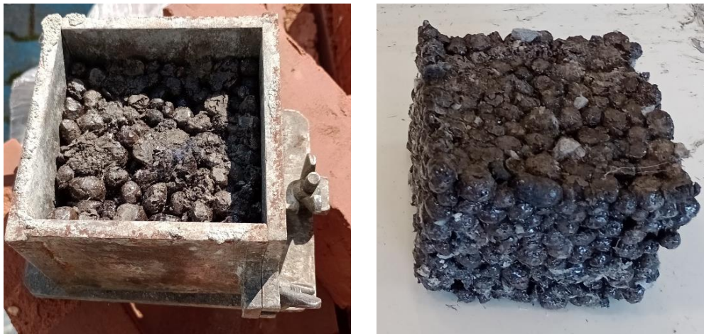
Fig. 3: Filling the mold for sample production (left) and the created test sample (right).
