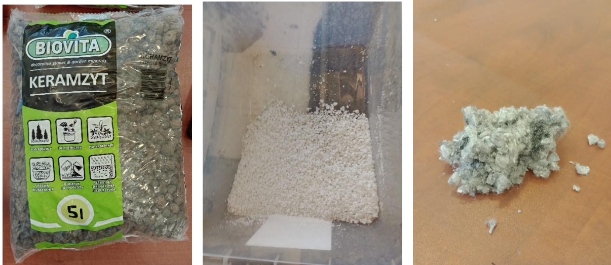
Fig. 2: Components of the test mixture: Liapor fraction 8/16 mm (left), EPS beads (center), and polyester fibers (right).
