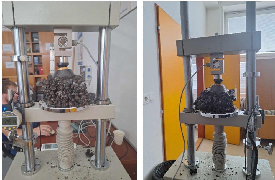
Fig. 5: Demonstration of sample collapse during the compressive strength test.
