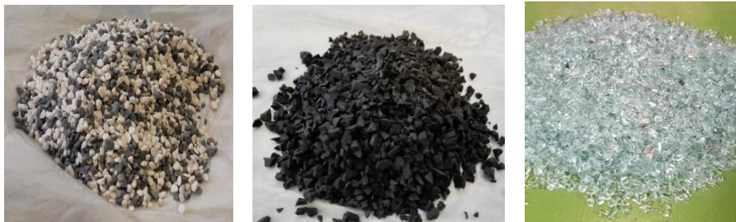
Fig. 1: Course materials (Left) aggregate (middle) crushed rubber (Right) crushed glass.
