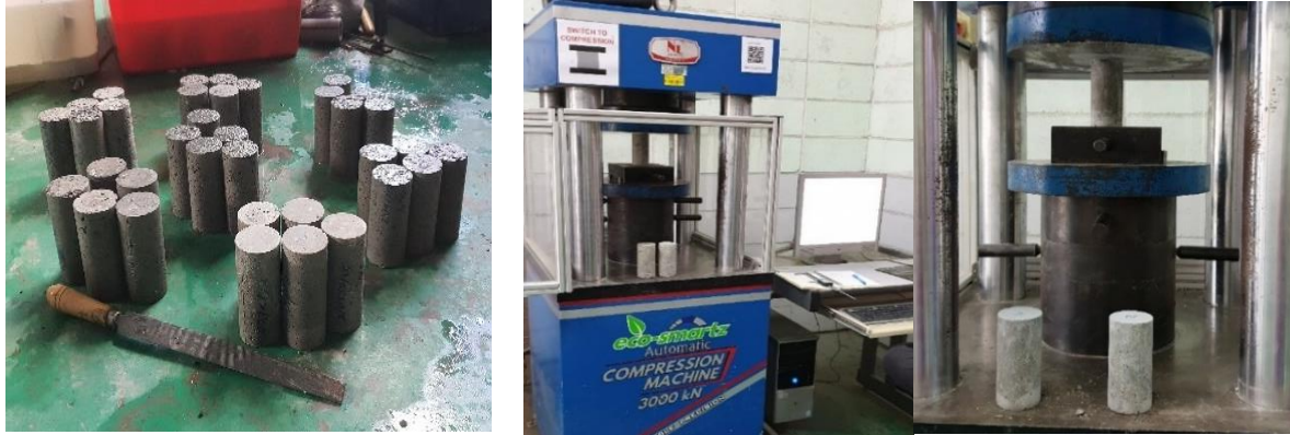
Fig. 3: Compressive strength test (left) prepared cylinders (right) testing machine.
