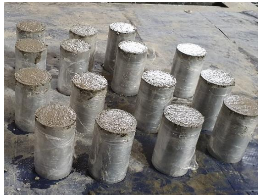
Fig. 2: Micro-concrete cylinders casting.
