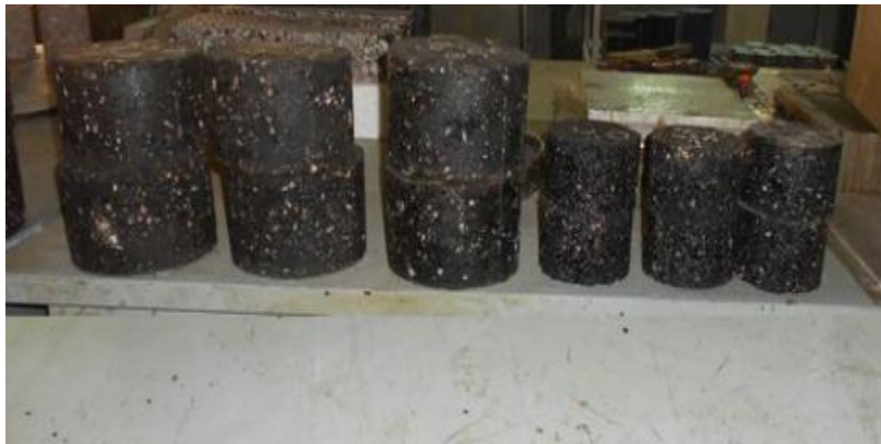
Fig. 2: Samples for optimum bitumen content (OBC).
