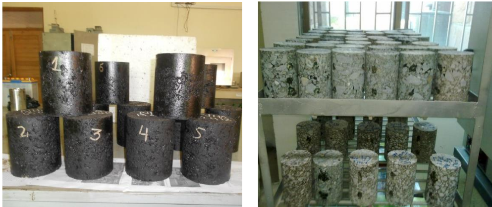
Fig. 3: Samples for dynamic modulus test.
