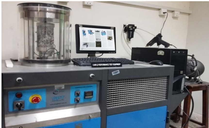
Fig. 4: Execution of simple performance test on cored sample.
