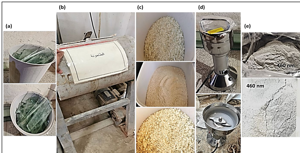
Fig. 2: Preparation process of Recycled Glass Powder.
