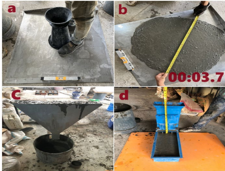
Fig. 3: Compatibility test progress (a) Slump Flow, (b) T500, (c) V-funnel, and (d) L-Box.
