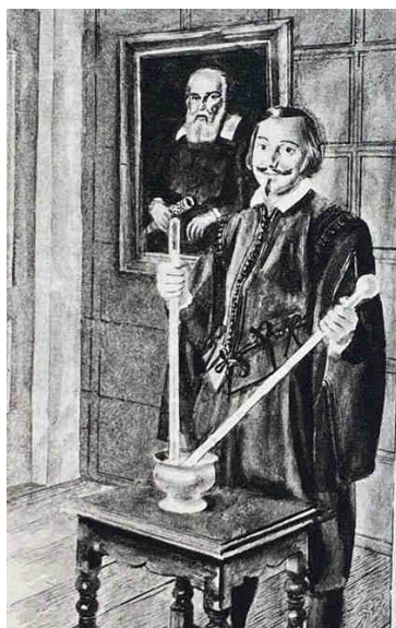
Fig. 3. "Torricelli demonstrates the vacuum. When the upper ends of the tubes are raised to the vertical, the mercury, which originally filled them, remains approximately 30 inches above the surface of the mercury in the bowl, leaving an empty space, which when the tube is lowered once more becomes filled with mercury" [10]
