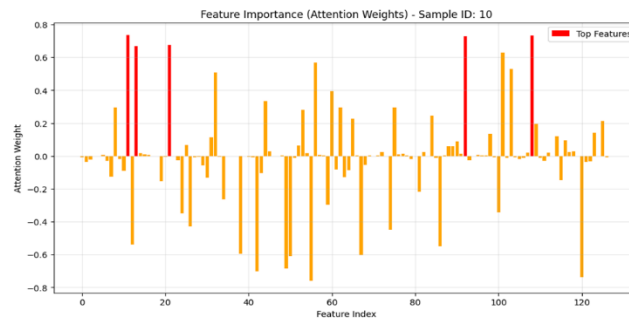
Fig. 7. Attention weight distribution for features at the sample level (Sample ID: 10). The red bars indicate the most influential features attended by the model for making the classification decision, reflecting local interpretability
