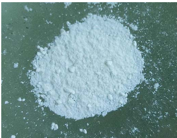
Figure 3. Glass powders obtained by the sol-gel method, after the heat treatment applied to the xerogel at a temperature of 600 °C
