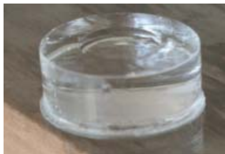
Figure 2. Gel sample aged for 54 hours at 60^\circ\text{C}
