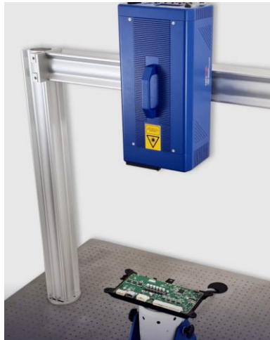
Fig. 2 – Scanning LDV experimental setup: vibrometer head and electrodynamic shaker.
