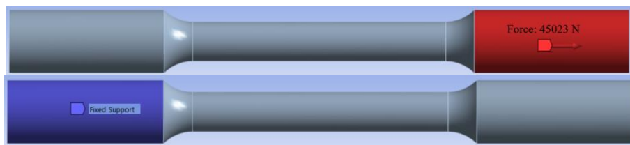
Fig. 13 – Boundary and loading conditions for a 10 mm diameter sample.
