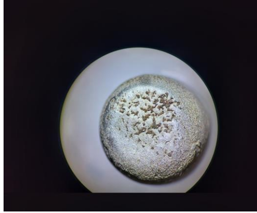
Fig. 12 – C-ECM processing using a 5% NaCl electrolyte at 10 V and a current density of 10–20 A/cm 2 .
