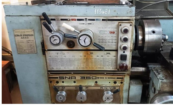
Fig. 5 – A front view of the mechanical gearbox of a lathe, used as driven mechanical system (running in idle).
