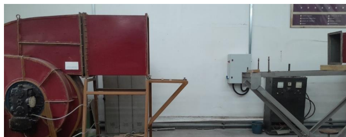
Fig. 3 – The MF-TA2 wind tunnel after removing the mentioned components (Pavăl, 2024).
