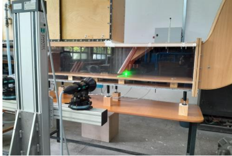
Fig. 15 – Image of the Laser Doppler Anemometer during the experiments (Pavăl, 2024).
