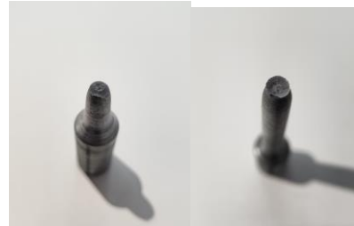
Fig. 4 – Typical ductile fracture appearance for OLC45 steel.
