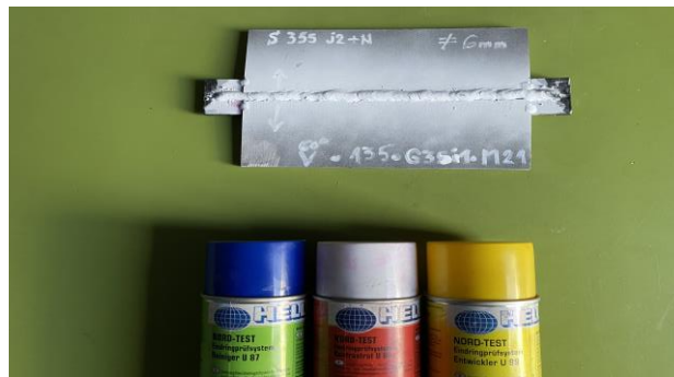
Fig. 4 – Penetration liquid was applied to the welded joint part.
