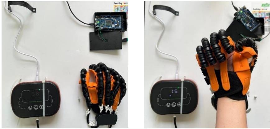
Fig. 3 (a), (b) – The Developed System for Experimental Data Collection Using the Pneumatic Glove.
